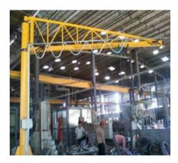
Jib Cranes are useful where the material needs to be loaded & unloaded with in a small area such as machining work station, truck loading unloading bay, finished product packing etc. Jib cranes can be provided either in standalone module or wall mounted module. The rotation of the arm (Boom) can be upto 3600. The arm (Boom) radius can be upto 6 meters.
